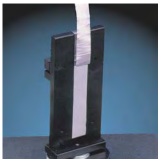
180° Flexible/Rigid Substrate Peel Test
