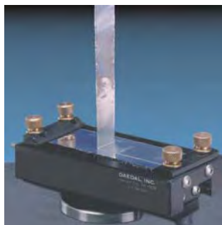
90° Rigid Substrate Peel Test
