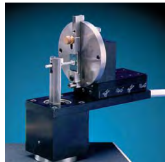
Tipple Tear Test
