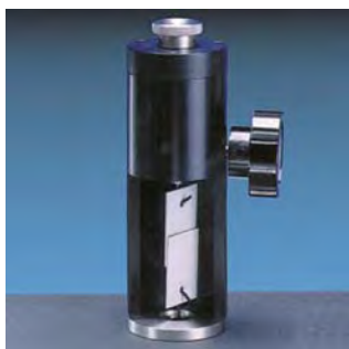
Tensile Breaking Point Test
