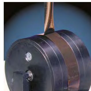
90° Flexible Substrate Peel Test
