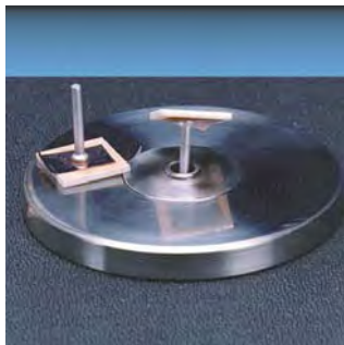
Stud Pull Coating Adherence Test
